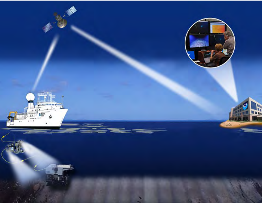
NOAA Ship Okeanos Explorer uses satellite and Internet2 technologies to transmit data and video in real-time from the ship and ROVs at depth, to audiences ashore, including scientists at exploration command centers. The University of Rhode Island's Inner Space Center compresses the video for distribution via standard Internet. Video and internet-based collaboration tools allow scientists on shore to join the expedition in real-time. Credit: B. Ambrose, GDIT/NODC, R. Canfield, NOAA & NOAA OER.
