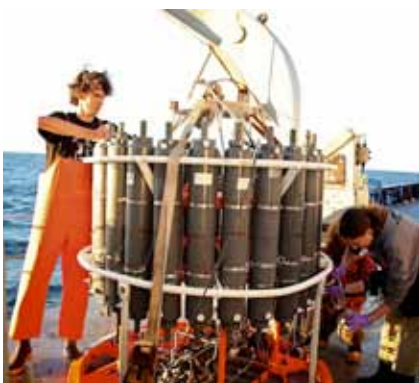
Ben Grupe begins to prepare the CTD bottles for deployment, an instance when being tall comes in handy. Normally, scientists have to climb onto the white frame to cock the bottle caps. As the CTD is lowered into the ocean, a computer is used to watch the data and order bottles to snap shut, collecting water samples from different depths. Photo courtesy of INSPIRE: Chile Margin 2010.
