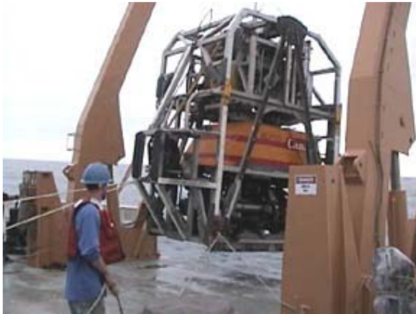
ROPOS being deployed for deep water operations inside its steel cage.
