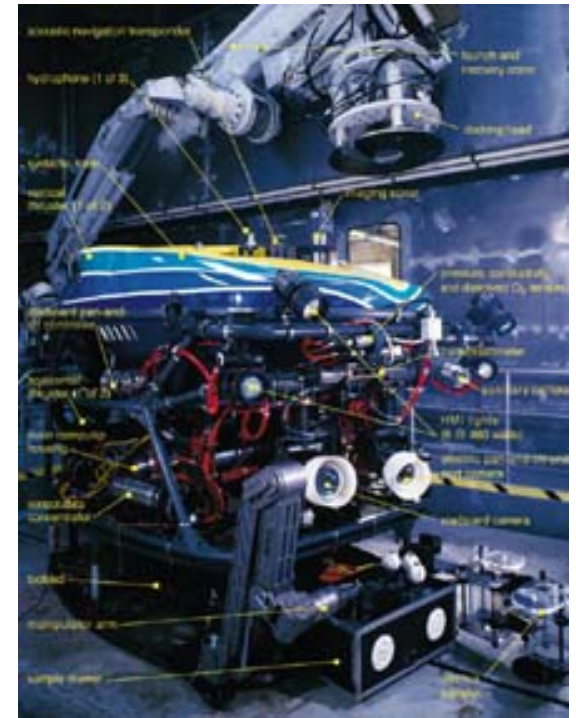
Sensors and sampling tools on the Tiburon. Photo: MBARI
