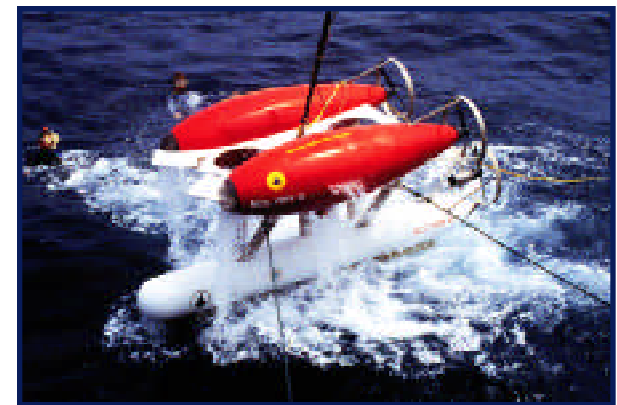
Autonomous Benthic Explorer known as ABE. Photo courtesy of Woods Hole Oceanographic Institution
