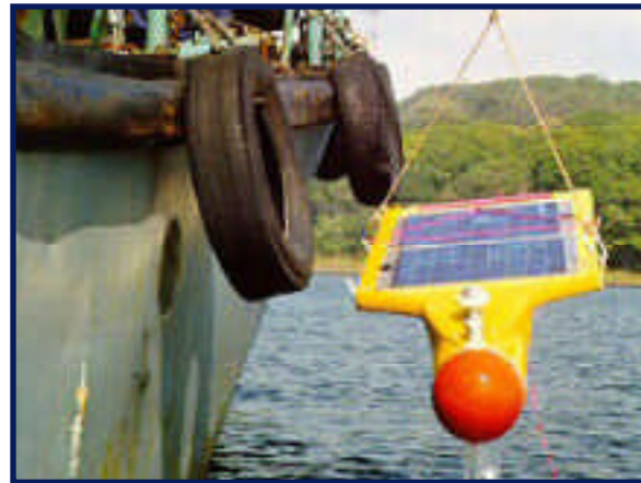
The Solar Powered AUV (SAUV) being retrieved after sea test off Vladivostok. This extremely long endurance AUV is part of a joint development effort between the Institute for Marine Technology Problems (IMTP) in Vladivostok, Russia, and the Autonomous Undersea Systems Institute in Lee, New Hampshire. Photo courtesy of the Autonomous Undersea Systems Institute
